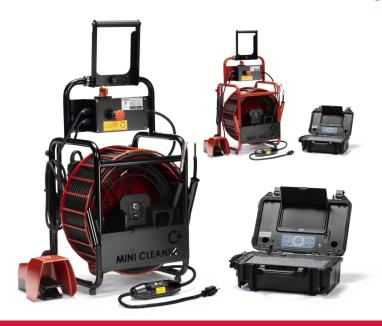
The Picote Mini Miller +C and Mini Cleaner +C units feature an integrated 30m (98') color camera that makes viewing of cleaning and cutting jobs easier and helps to make Picote Brush Coating™ setup even simpler.
