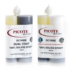
**Re-coat** - 3 hrs at +21 °C / +70 °F **Restore flow** - 4 hrs. **Final Cure** - 24 hrs. Can be recoated within 12 hrs with no prep, <u>grinding panels must be used after 12 hrs</u>. **Installation:** +10 °C / +50 °F to +60 °C / 140 °F **Storage:** Room Temp +16 °C / +60 °F to +29 °C / +85 °F
