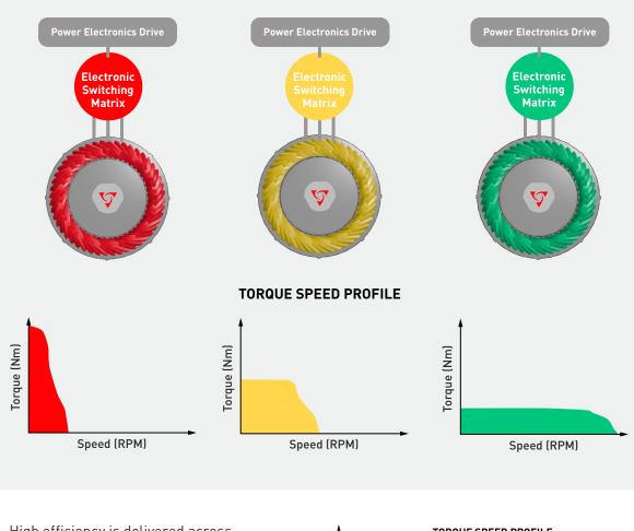
High efficiency is delivered across a greater range of the torque/speed profile.
