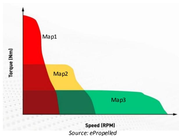
While an electric motor is inherently more efficient than an IC engine, the efficiency maps are similar. Typically, the highest efficiency is for a specific combination of torque and rpm. Moving away from this combination reduces the efficiency of the electric motor.
