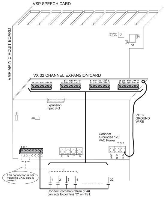
Electrical Connection Diagram For Dry Contact Inputs
