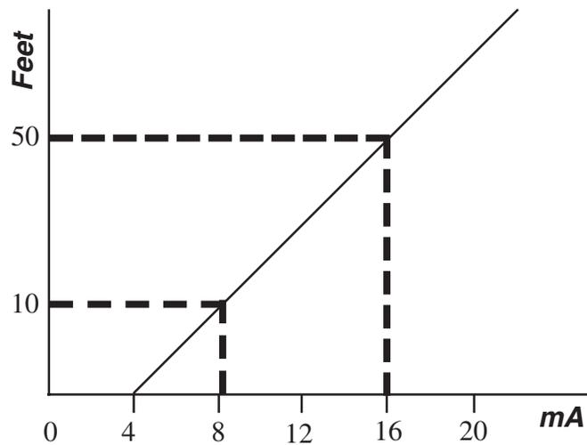
where  $m$  is the gain and  $b$  is the zero crossing point or Input (ma  $\rightarrow$  offset). The gain may be calculated from:  $m = (y_2 - y_1) / (x_2 - x_1)$
