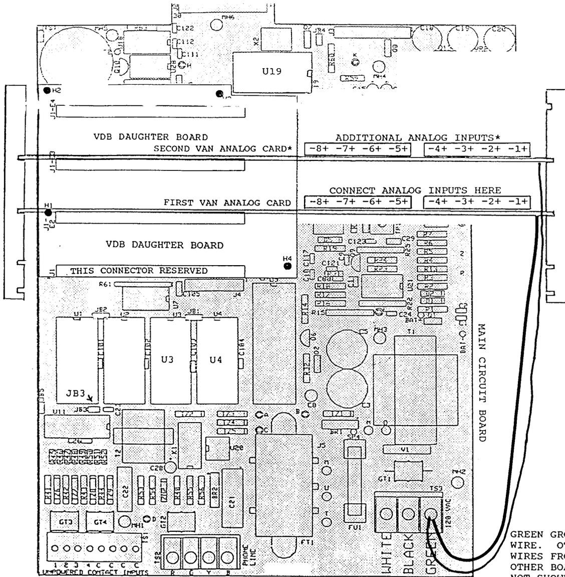
\*UNITS EQUIPPED FOR 16 ANALOG CHANNELS WILL REQUIRE 2 VAN CARDS. THE SECOND (UPPER) CARD WILL BE FOR THE HIGHER NUMBERED ANALOG CHANNELS. THE SECOND VAN CARD IF ANY WILL HAVE ITS JB50 JUMPER STRAP IN THE UPPER POSITION.
