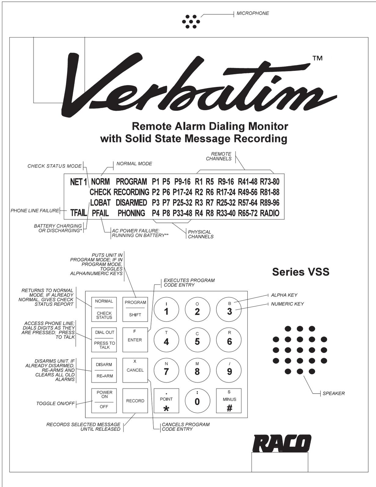
\* A discharged battery may take up to a day to fully charge. \*\* During AC power failure, all illuminated LED's will flash to conserve battery power. Meanwhile, light may remain on.
