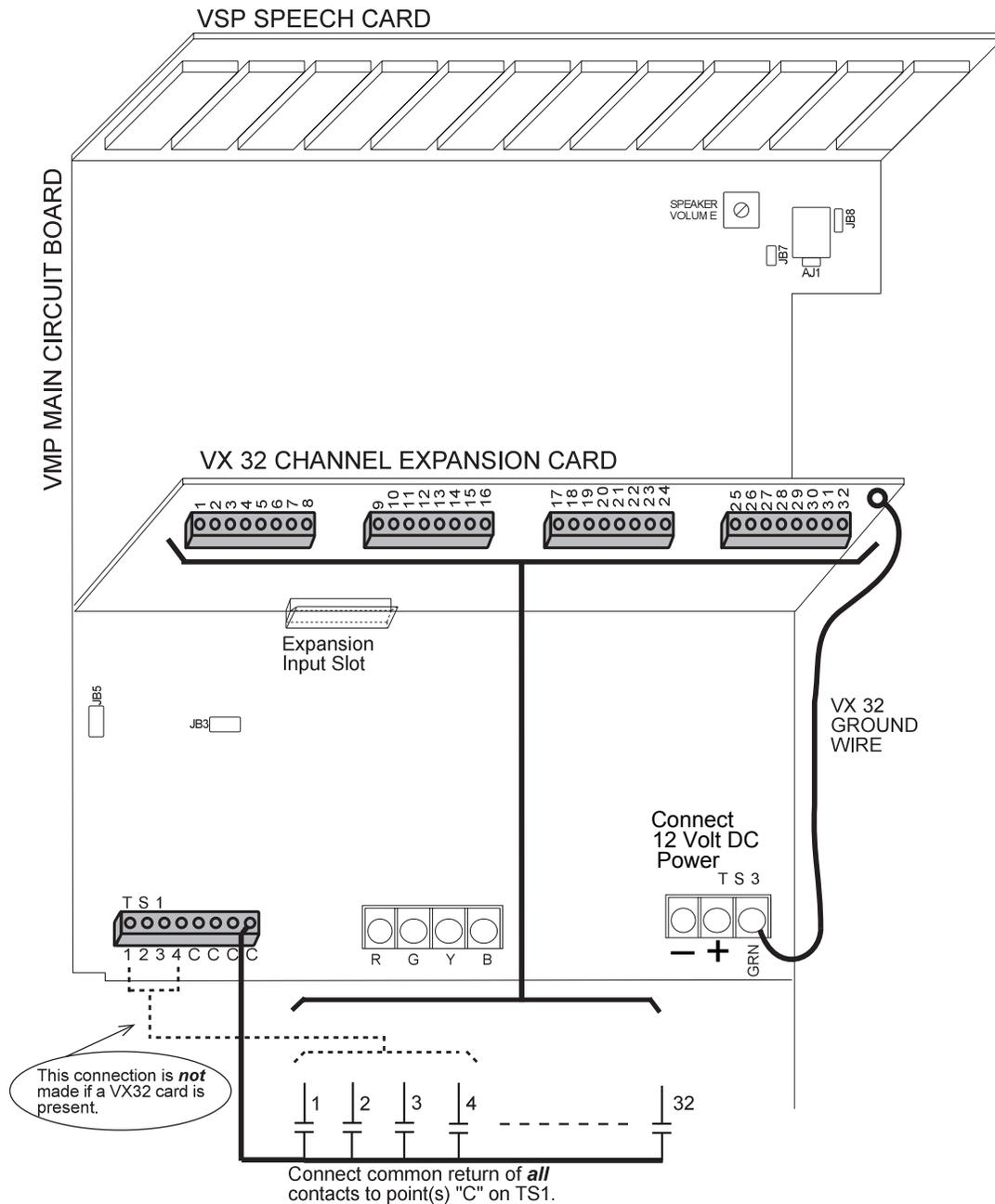
The common returns for all inputs are connected to TS1 terminals marked "C". These four "C" terminals are connected together and to electrical ground.
