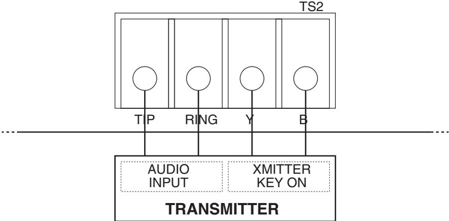
*Jumper Wires For RF Link Diagram*
