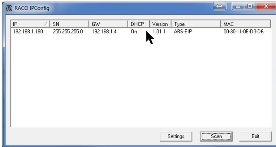
3. If more than one *Gateway* is found, you may need to temporarily disconnect one or more of them to determine which the correct one is. Alternatively, you can compare the MAC address printed on the Ethernet module to the displayed MAC.
