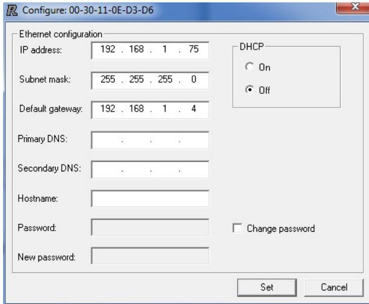
5. It is highly recommended that the *Gateway* and PLC be assigned static IP addresses to avoid loss of connectivity if the DHCP server assigns a different IP than the system was configured to use.
