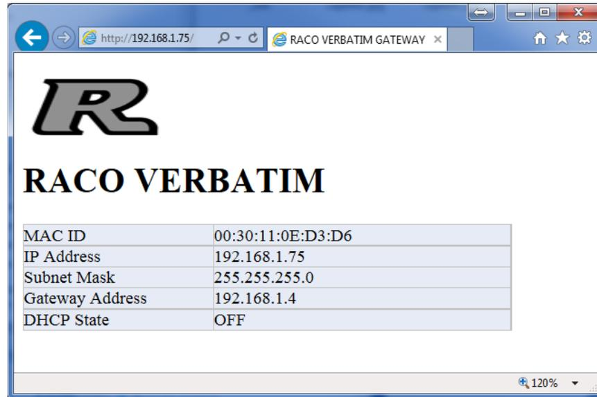
The Gateway Ethernet Module is now configured and ready to receive data from other devices on the network.
