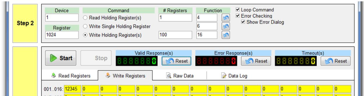
11. **Click Start.** Observe the *Alarmware Direct Channel Reading* window. The **Raw value** should equal the same number that was entered in the *ComTest Pro* register. The **Report Value** applies any scaling that has been added; we had entered a gain of 2 in this example. See the *Gateway* manual for information on scaling and other aspects of the channel setup.
