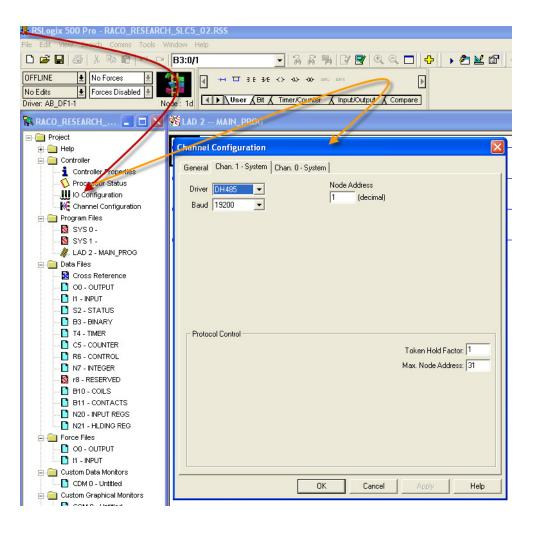
The following seven-step procedure will configure your Verbatim Gateway to link its Remote Channels (RC) to your PLC via DH485. Once linked, the Verbatim Gateway will monitor RC status and Alarms according to your settings.
