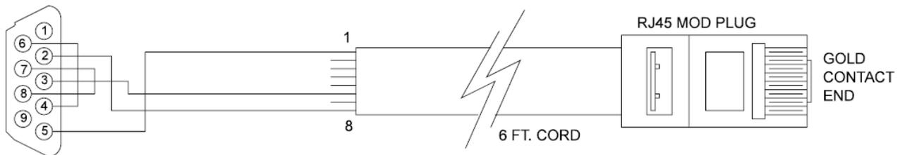
9 Pin Connector Pin-Out
