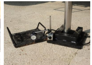
Float & dial gauge for monitoring settlement
