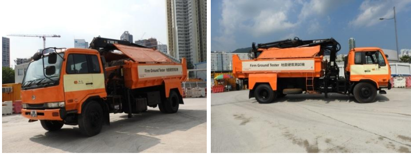
Firm Ground Tester – A designated truck equipped with a set of hydraulic jack and measurement devices for load and settlement
