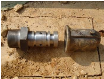
A jet lock pre-welded to the toe of SSP for engagement of water nozzle
