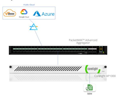
Garland Technology has exclusively partnered with Nubeva for traffic capture in the cloud, so corporate traffic in public cloud environments including AWS, Google Cloud Platform, and Azure can be captured via a Nubeva Prism, transmitted to Garland, and then streamed to a Corelight Sensor to be transformed into logs, extracted files, and security insights.
