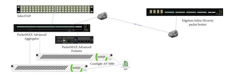
The scalable design of multi-network environments with satellite locations allows for easy deployment and management of remote sensors along with other monitoring and inline devices. At the primary location, Garland's SelectTAP™: Fiber Modular Chassis is tapping multiple links, sending traffic through the PacketMAX™ Advanced Aggregator for aggregation and the PacketMAX Advanced Features box for deduplication.
