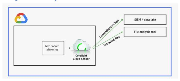
The Corelight Cloud Sensor deploys as a GCP VM image instance and ingests traffic directly via GCP Packet Mirroring or from 3rd party packet-forwarding agents. With a few simple config changes, the sensor will export data to downstream storage and analytics tools such as SIEMs or file analysis platforms.
