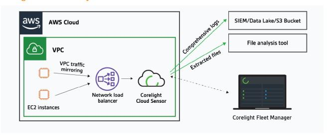
The Corelight Cloud Sensor can ingest traffic via Amazon VPC traffic mirroring (enabled per EC2 instance) or via an Amazon Network Load Balancer, streaming logs and extracted files to SIEMs, Amazon S3, or file analysis tools. Customers can fork and filter the data via Corelight's management console and easily manage multi-sensor environments with Corelight Fleet Manager's sensor policy templates and role-based access controls.
