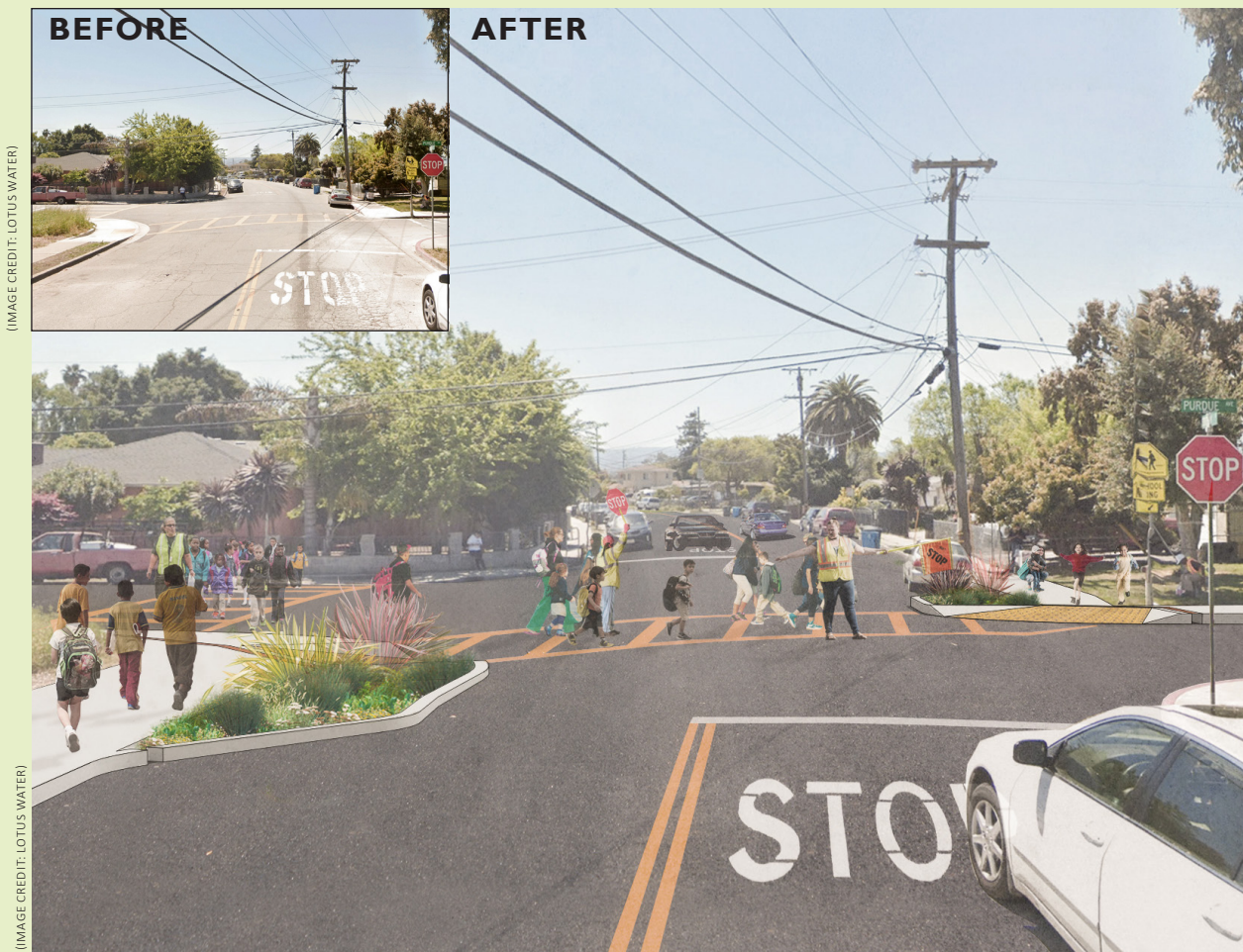
Figure 4-3: This before and after sequence shows how a sustainable street curb extension can shorten pedestrian crossing distance and provide stormwater management and neighborhood greening near a school in East Palo Alto.
