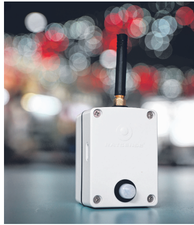
Ratsense's infrared motion sensors can help detect rodent presence via a change in temperature in an area.
