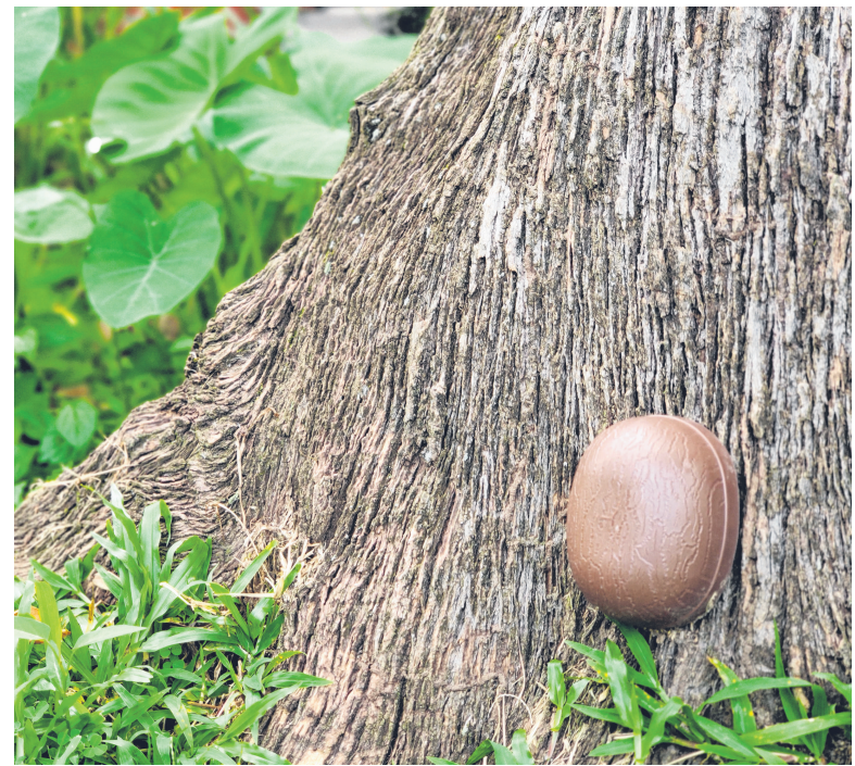
A tilt tree sensor installed by technology company Styl Solutions at Bishan-Ang Mo Kio Park as part of a pilot by the National Parks Board in the first quarter of last year. PHOTO: STYL SOLUTIONS
