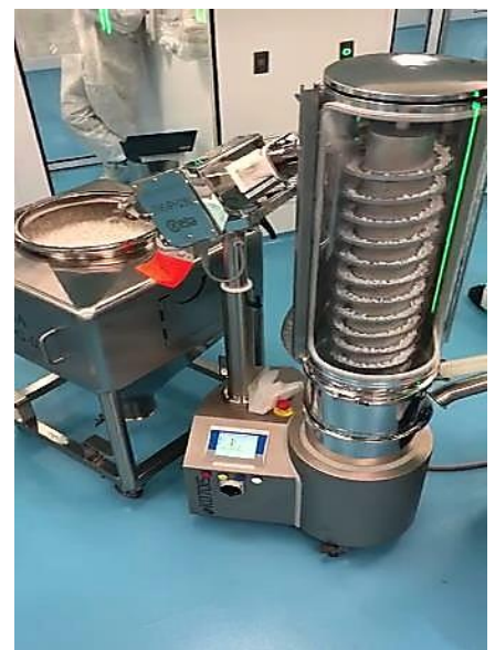
Pharma Plant Solid Products process with direct compression
