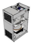
Put back the process fan top cover and fix the screws.
