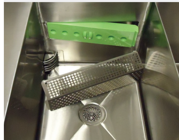
Removable Wash Jet Channel & Wash Pump Intake
