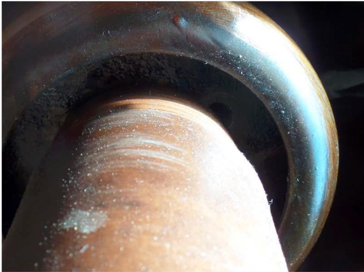
N phase – heat decolourisation markings of corona shield with some pitting
