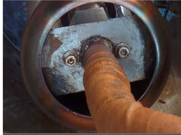
N phase – Heat decolourisation markings of corona shield with some pitting. Brittle paper pieces seen plus paper has voids from incorrect laying.
