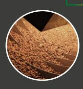
The material is conveyed uniformly through the machine by means of the spiral screw at variable turning speed, and simultaneoulsy heated with infrared light. When necessary, water or other liquids can be added to the product during treatment.
