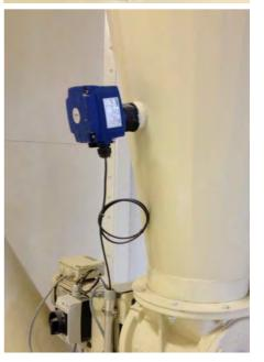
In order to handle the extremes in temperature, UWT has integrated small heating elements into the electronics of their measuring instruments. Thus, the sensor is carefully adjusted to the dramatic change in temperature, which allows accurate switching circuit without the result being adversely affected.
