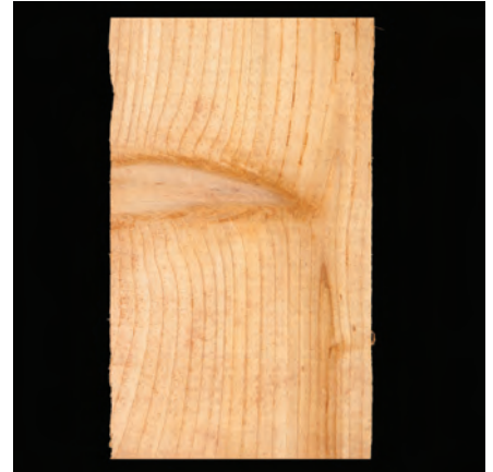
Spike knot — A knot created when a limb is sawn either lengthwise or diagonally across the face of a piece of lumber.
