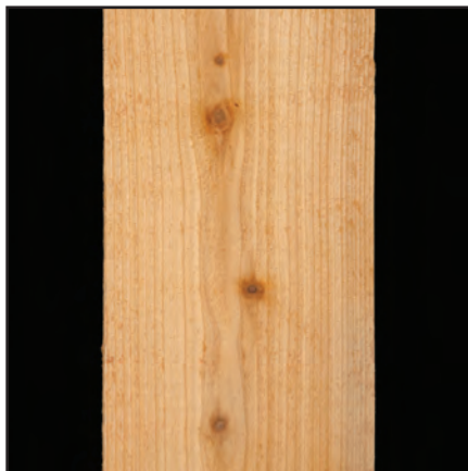
Pin knot — A small knot or grain swirl.
