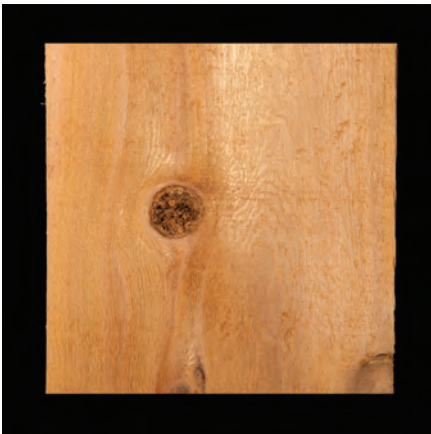
Unsound (soft) knot — A knot that keeps its position, but contains decay or is soft to the touch.
