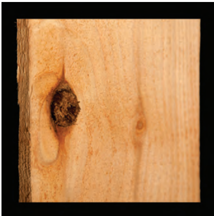
Loose knot — A knot that will not keep its position in a piece of sawn lumber.
