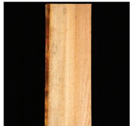
Wane — The lack of wood fiber on the edge or corner of a piece of lumber.
