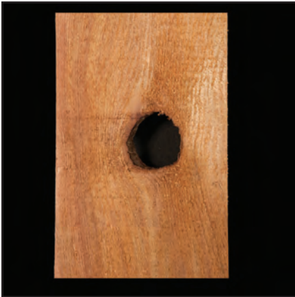
Thru hole — A section of lumber that is void of fiber wholly through the piece. The most common cause of thru hole is from the loss of a knot.
