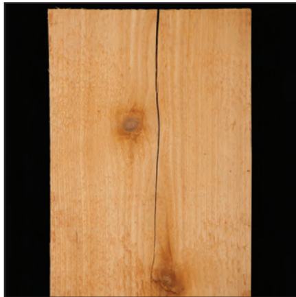
Split — A separation of wood through the piece to the opposite surface, caused by the tearing apart of the wood cells.
