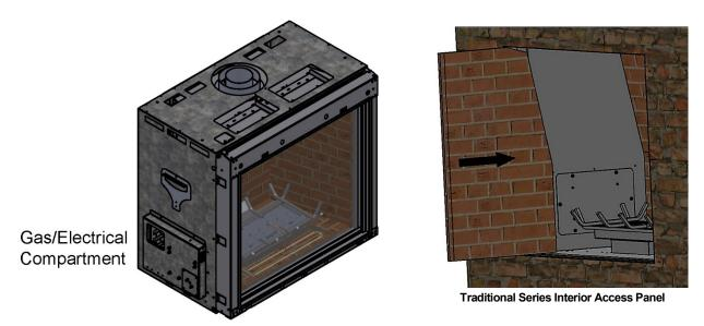
An access panel is not required (see notes below for exception), but it is <u>highly recommended</u>. It allows for access to the fireplace's gas and electrical components for servicing.
