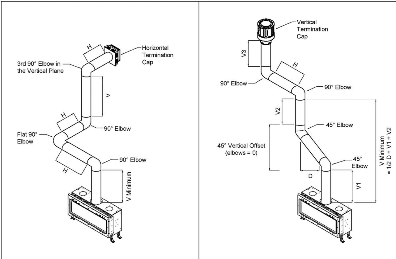
**! TERMINATION CAP NOTE:** Low Profile Vertical Termination Cap and Sconce Horizontal Termination Cap can negatively impact flame appearance and are not recommended for use with the fireplace.
