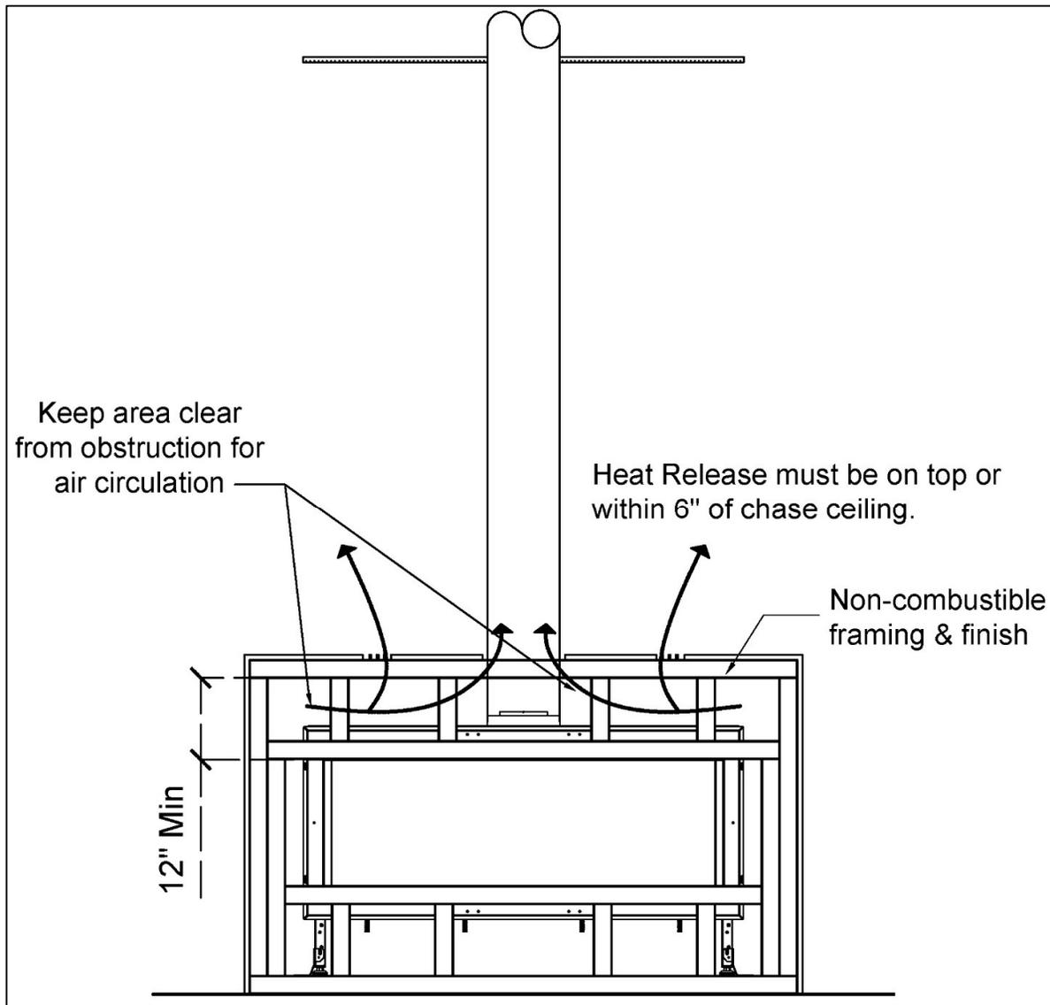
Minimum Chase Ceiling Clearance Diagram
