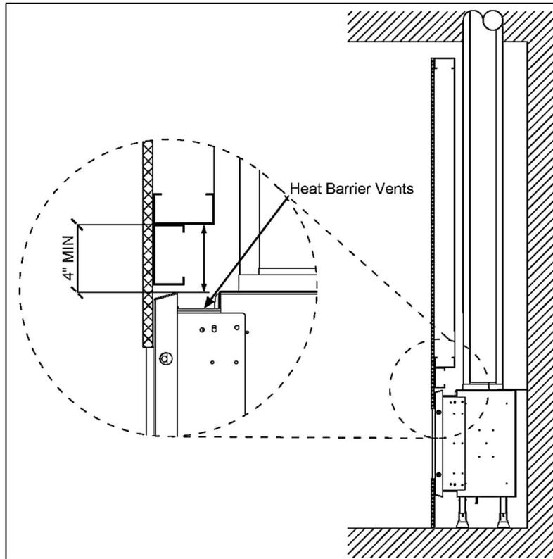
**!** NOTE: It is acceptable if the flat stud immediately above the fireplace hangs over heat barrier vents *slightly* when using standard metal framing (as shown in diagram above).
