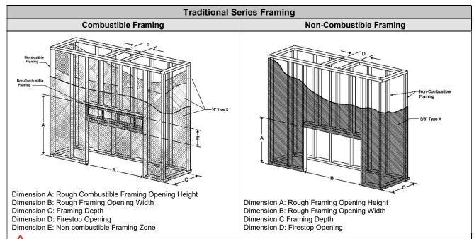
WARNING – MAINTAIN AIR FLOW CLEARANCE: Firebox top vent must have minimum 4" of clearance to any material achieve sufficient airflow. Failure to do so could result in improper fireplace operation, property damage, or physical injury. Review "General Clearances" section prior to framing to ensure all clearances are followed.
