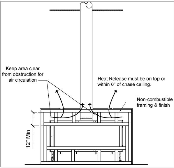
Minimum Chase Ceiling Clearance Diagram
