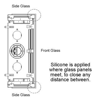
Glass Seal Assembly Diagram
