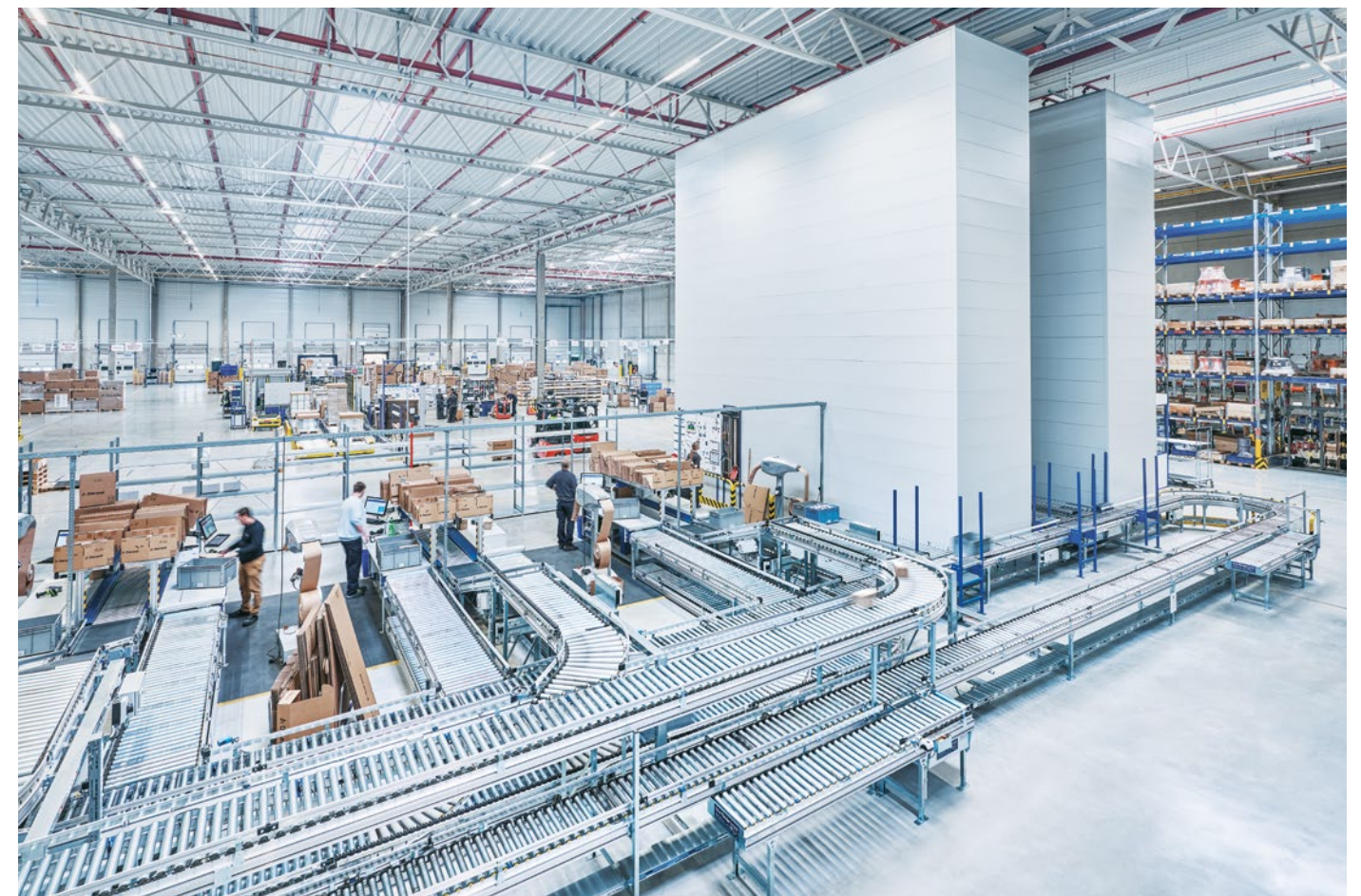
Vertical Buffer Modules LR 35 with automated conveyor connection
