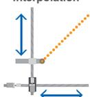
Movement is made in a linear line shape synchronizing the 2 orthogonal axes.
