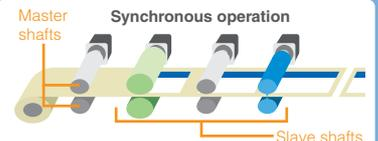
The slave shafts operate in conjunction with the movement of the master shafts.
