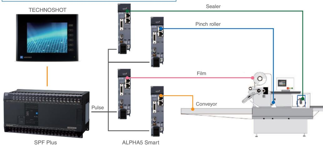
The film, conveyor, pinch roller and sealer operate synchronously with the operational pattern being automatically calculated from the length of the cut.
