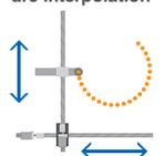
Movement is made in a circular arc shape synchronizing the 2 orthogonal axes.
