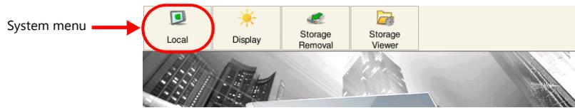
2. Press the [Local] switch on the system menu. The Local mode screen is displayed on the unit.
