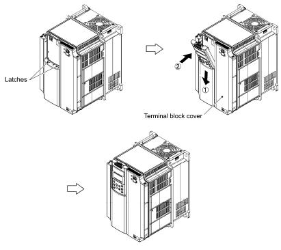
Figure 2.3-5 Mounting the Keypad
