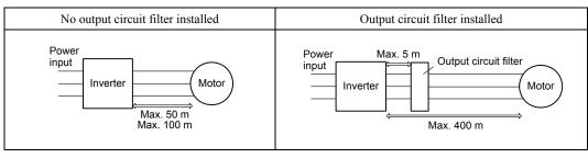
If using the motor with encoder, 100m below the wiring distance between the inverter and the motor. This is due to the limitation on the specifications of the encoder. If it exceeds 100m, the action is required, such as in the middle put the isolated converter.
