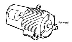
Figure 4.2-2 Forward Rotational Direction of Motor and PG
