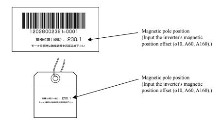
Figure 4.4-2 Magnetic Pole Position Offset Labels
