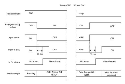
Figure 8.4-5 ELF Alarm (Caused by Logic Discrepancy) and Inverter Output State
