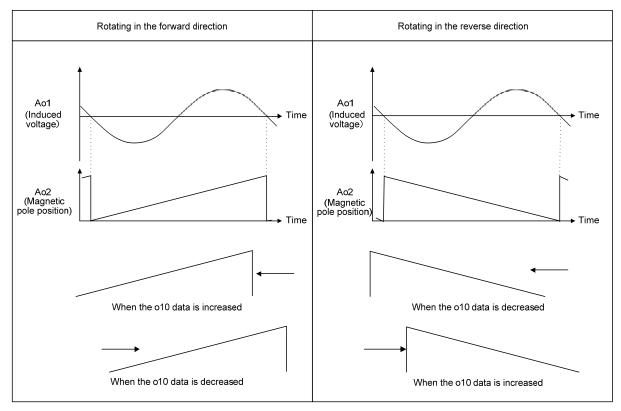
Figure 4.4-3 Adjustment of Magnetic Pole Position
