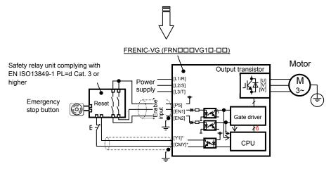
\*Transistor output terminals (e.g., [Y1]-[CMY], *DECF* (Function code data=80), Refer to Section 5.3.)
