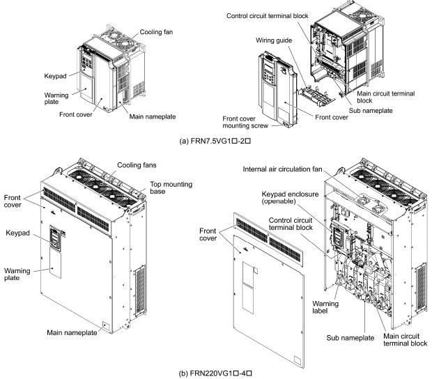
Figure 1.2-1 Outside and Inside Views of Inverters
