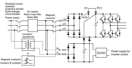
Figure 2.2-3 Connection Example of Residual-current-operated Protective Device (RCD)/ Earth Leakage Circuit Breaker (ELCB)
