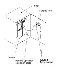
Figure 2.3-2 Mounting the Keypad on the Panel
