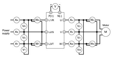
Figure 7.5-1 Connection of Meters
