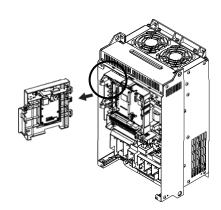
4) Fully insert the battery connector into the connector CN7 on the control printed circuit board.
