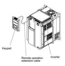
Figure 2.3-3 Using the Keypad Remotely in Your Hand
