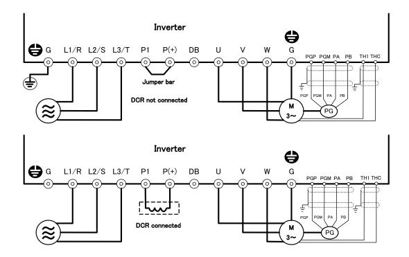
**Note:** In principle, the shielded sheath of wires should be connected to ground. If the inverter is significantly affected by external induction noise, however, connection to 0V may be effective to suppress the influence of noise.
