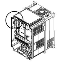
Fully insert the battery connector into the connector CN7 on the control printed circuit board.
