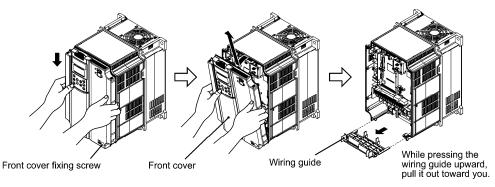
Figure 2.2-1 Removing the Front Cover and the Wiring Guide (FRN11VG1□-2□)
