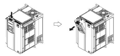
Figure 2.3-4 Removing a Keypad
