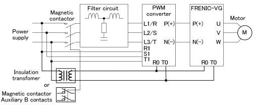
Figure 2.2-4 Connection Example of PWM Converter
