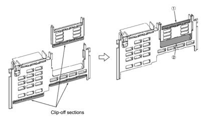
If the inverter output wire size is 22 mm<sup>2</sup>, remove clip-off section before wiring. If it is 38 mm<sup>2</sup>, remove clip-off section before wiring.
