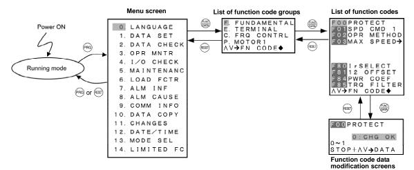
Figure 3.2-1 Configuration of Screens for "DATA SET"
