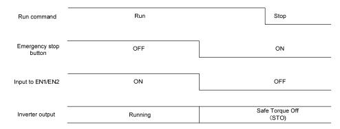
Figure 8.4-4 Inverter Output State when the Emergency Stop Button is Turned ON with the Inverter Running
