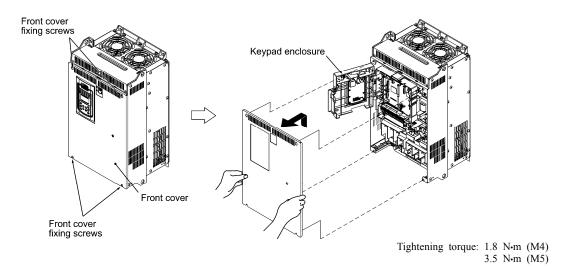
Figure 2.2-2 Removing the Front Cover (FRN30VG1□-2□)
