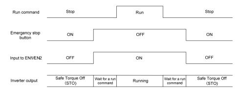
Figure 8.4-3 Inverter Output State when the Emergency Stop Button is Turned OFF with the Inverter being Stopped
