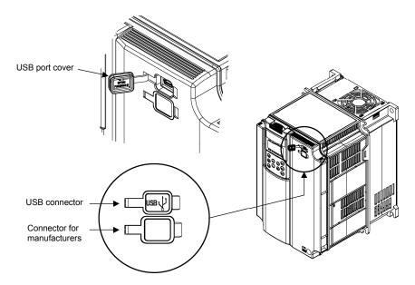
Figure 2.4-1 Connecting a USB Cable
