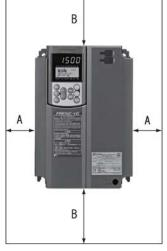
Figure 2.1-1 Mounting Direction and Required Clearances
