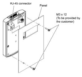
Figure 2.3-7 Mounting the Keypad
