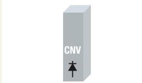
This converter is used where no electric power regeneration is required.
