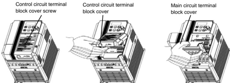
[ Removing the Terminal Block Covers ]
