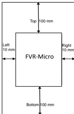
Figure 2.1 Mounting Direction and Required Clearances
