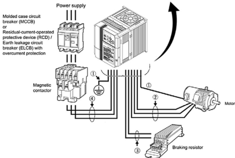
Figure 3.1 Wiring procedures for Peripheral Equipment
