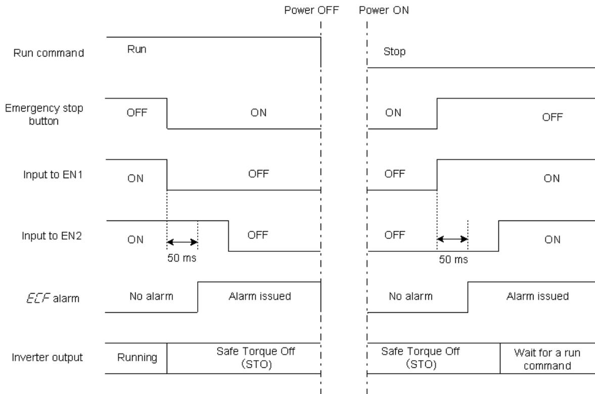
Figure 9.9 *EEF* Alarm (Caused by Logic Discrepancy) and Inverter Output State
