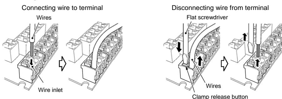
Table 2.7 lists the symbols, names and functions of the control circuit terminals. The wiring to the control circuit terminals differs depending upon the setting of the function codes, which reflects the use of the inverter. Route wires properly to reduce the influence of noise.
