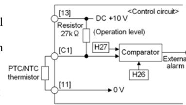
Figure 2.10 Internal Circuit Diagram (SW5 Selecting PTC/NTC)
