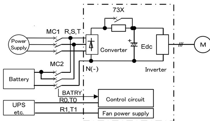
Figure B Connection Diagram
