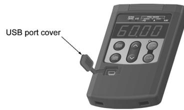
Connecting the inverter to a PC with a USB cable enables remote control from FRENIC Loader. On the PC running FRENIC Loader, it is possible to edit, check, manage, and monitor the function code data in real-time, to start or stop the inverter, and to monitor the running or alarm status of the inverter.
