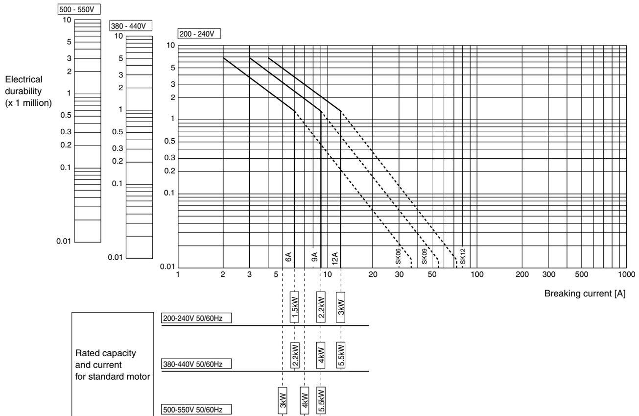
■ AC-1 Breaking Current and Electrical Durability
