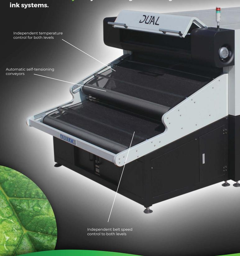
The Adelco Dual has a unique built in extraction system on the infeed and outfeed for a cleaner working environment together with independent exhaust extraction from each conveyor to maximize the curing efficiency for heavily water laden prints in both digital and conventional printing requirements
