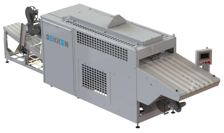
The **Dekken T-Apparel Pro III** offers automated textile folding and is designed to process hundreds of garments per hour. Built around the newest folding technologies offering automatic garment changes, it comes standard with a rear exit stacking unit and one by one rear exit. Optional features include a nose size labeler, post exit labeler, and bar code scanning for automatic recipe change over. Dekken offers affordable solutions for every size company from small to large scale manufacturing.
