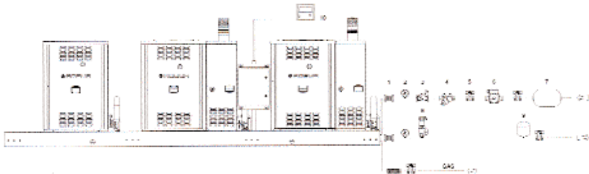
RTYF HYDRONIC SYSTEM: Typical Installation Arrangement for 2-pipe RTYF (External Components not included with Robur Unit)
