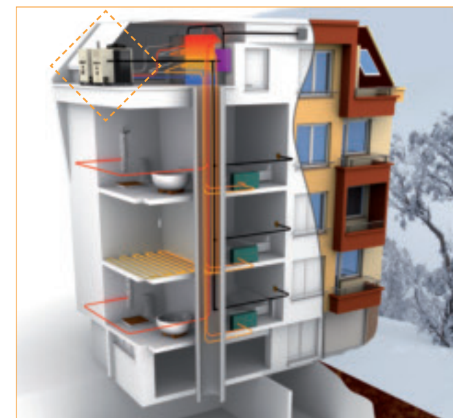
Example of GAHP-AR applications in winter and summer operation with radiant panels, fan coils and indirect production of DHW.
