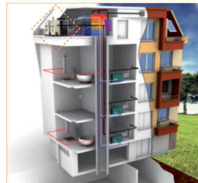
Example of GAHP-AR applications in winter and summer operation with radiant panels, fan coils and indirect production of DHW.
