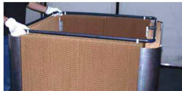
Figure 5.1 Cellulose evaporating panels
