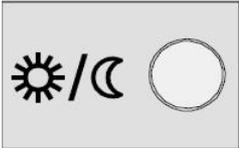
If, during heating in comfort mode, the rooms are unoccupied for a period of time, you can press the occupancy key L (fig. 3.1 p. 6) to switch to reduced mode and save heating costs.
