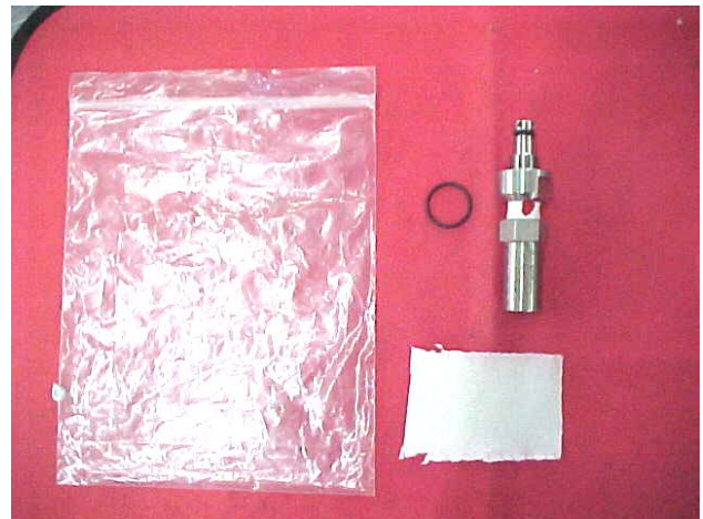
Figure 9.5 Safety valve kit - Components required for service
