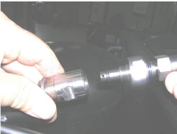
Figure 9.8 Removal of safety valve mobile part - Removal of safety valve
