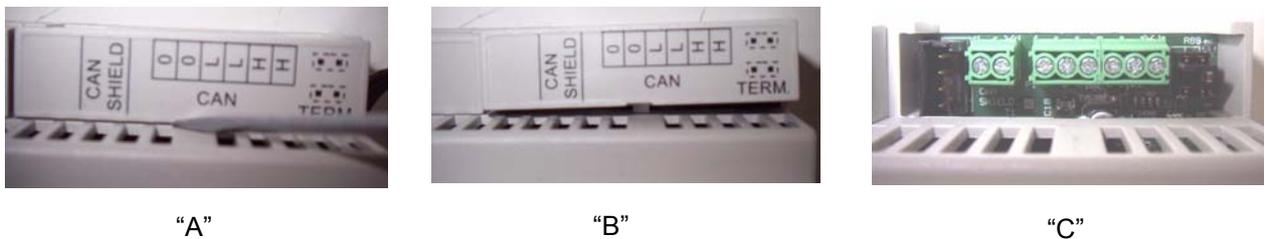
**Figure 25** Removing the CAN jumper cover (when necessary).
