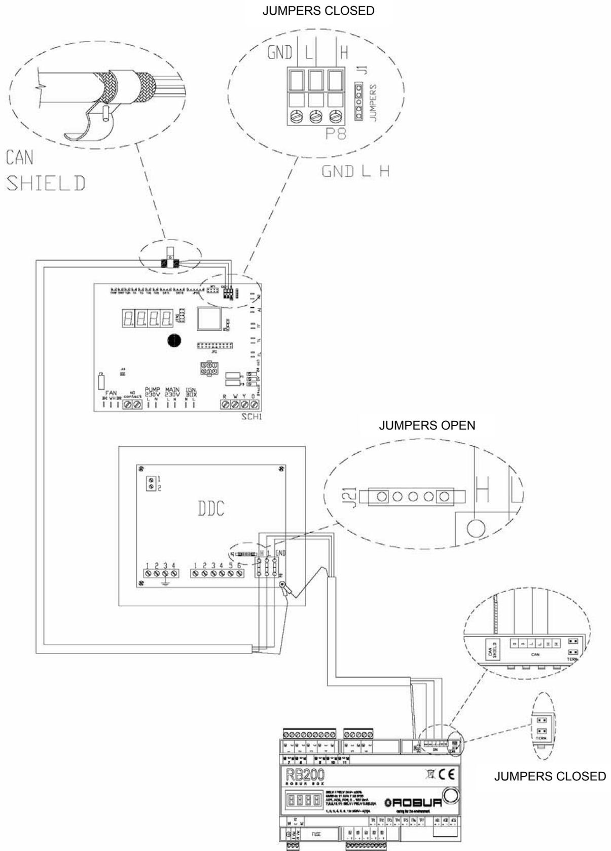
**Figure 26** Example of RB200 connection as final node.
