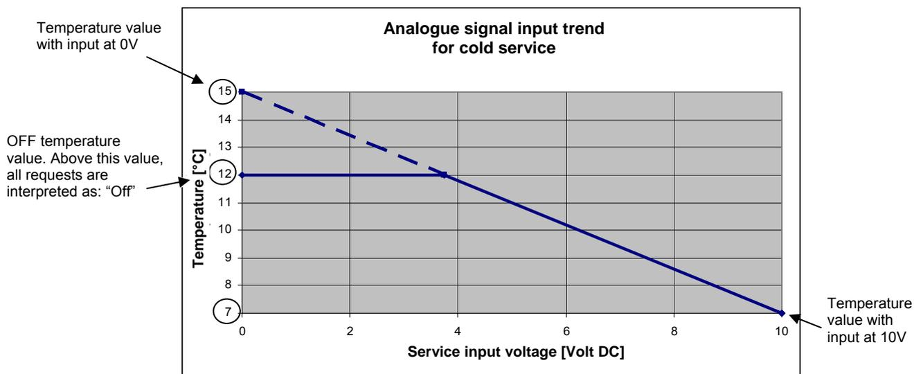
Figure 4 Voltage signal input trend for cooling analogue service
