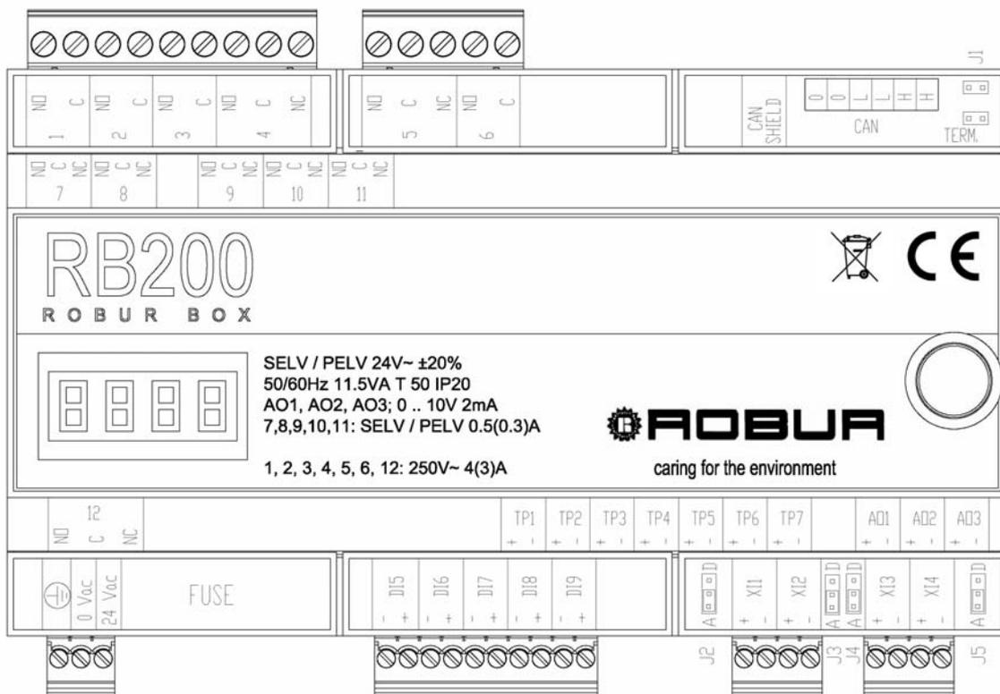
Figure 7 RB200 - representative diagram of the lower level connections
