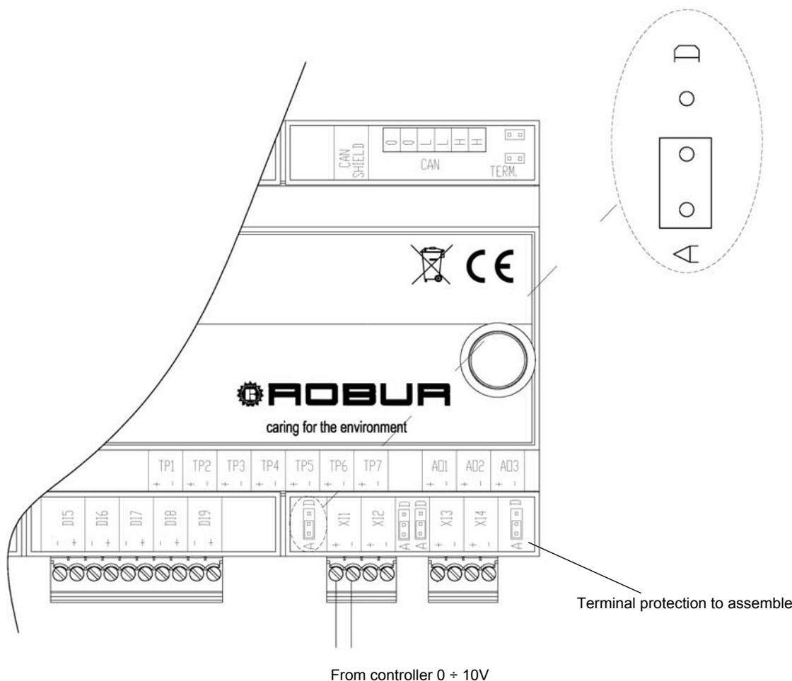
**Figure 10** RB200: electrical connection for analogue input
