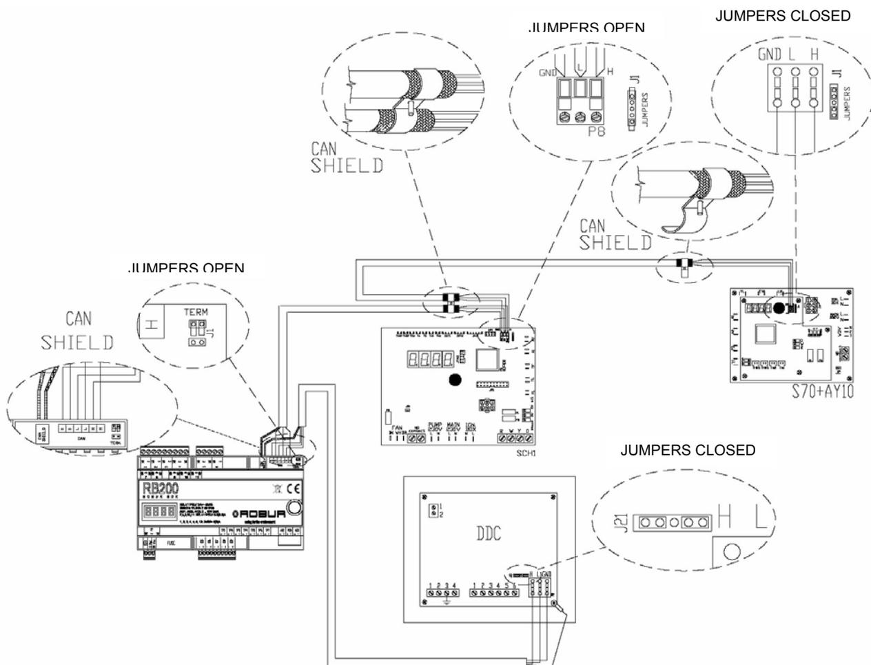
Figure 27 Example of RB200 connection as intermediate node.
