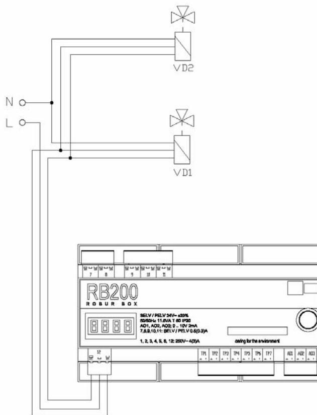
Figure 13 RB200: Example of electric connection for valve 2 service
