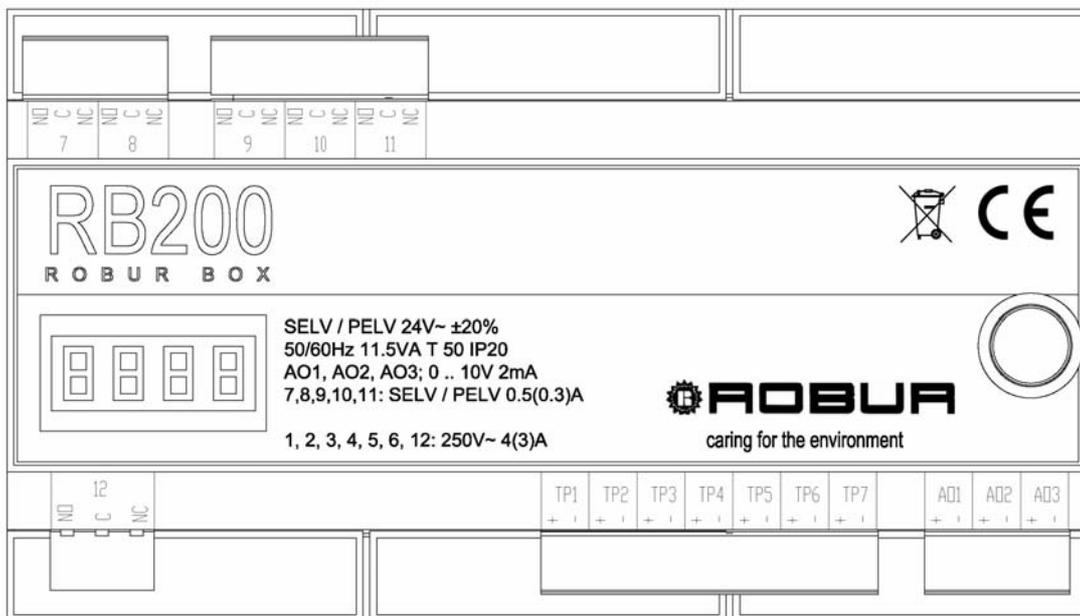
**Figure 8** RB200 - representative diagram of the upper level connections
