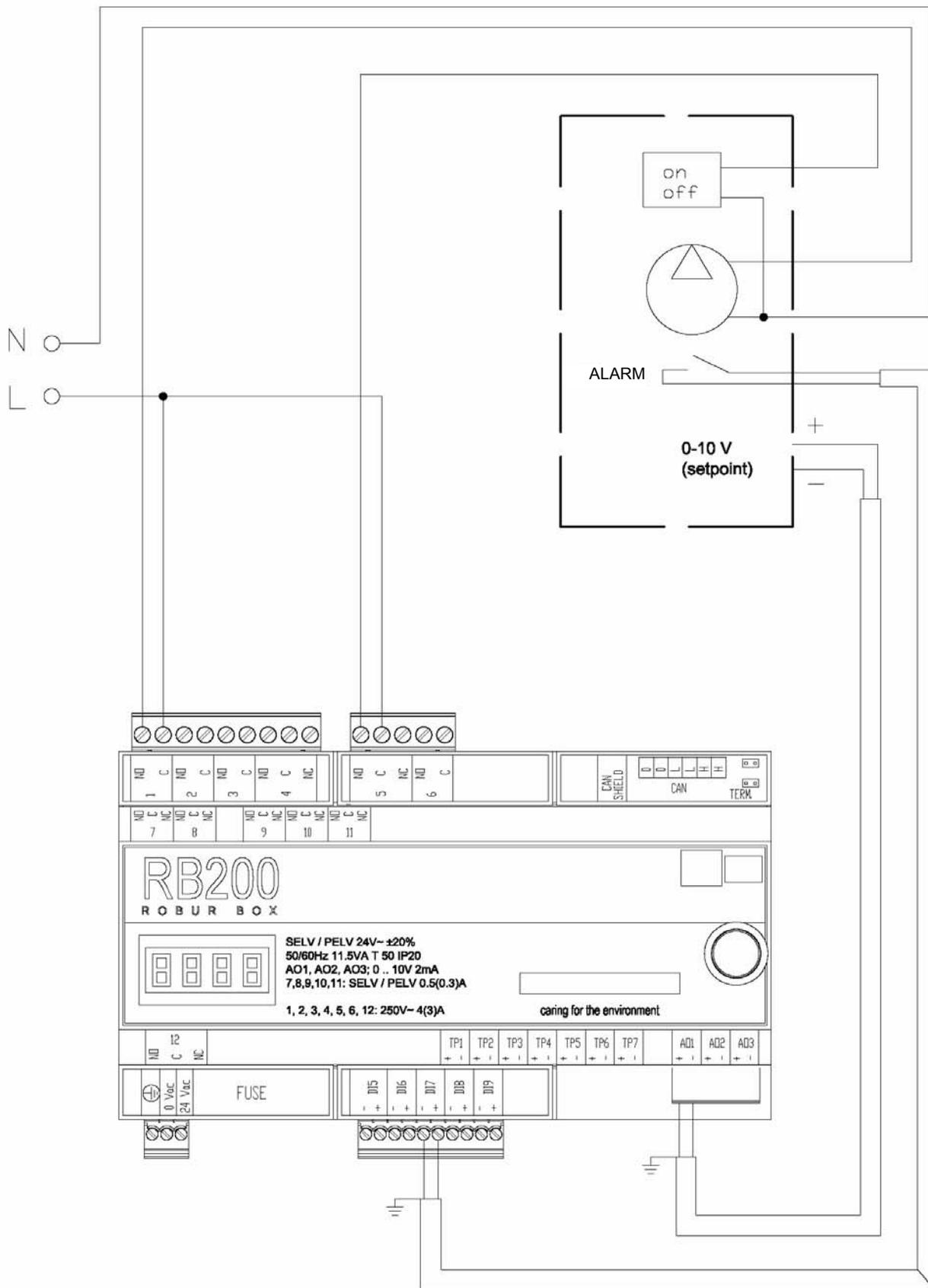
**Figure 14** RB200: Example of electric connection for generator 1 service
