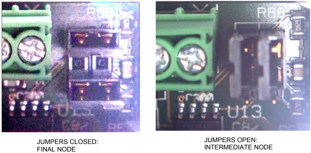
**Figure 24** JUMPERS PER FINAL NODE (FIRST PHOTO ON THE LEFT) AND PER INTERMEDIATE NODE (LAST PHOTO ON THE RIGHT): position recommended for OPEN jumpers highlighted.
