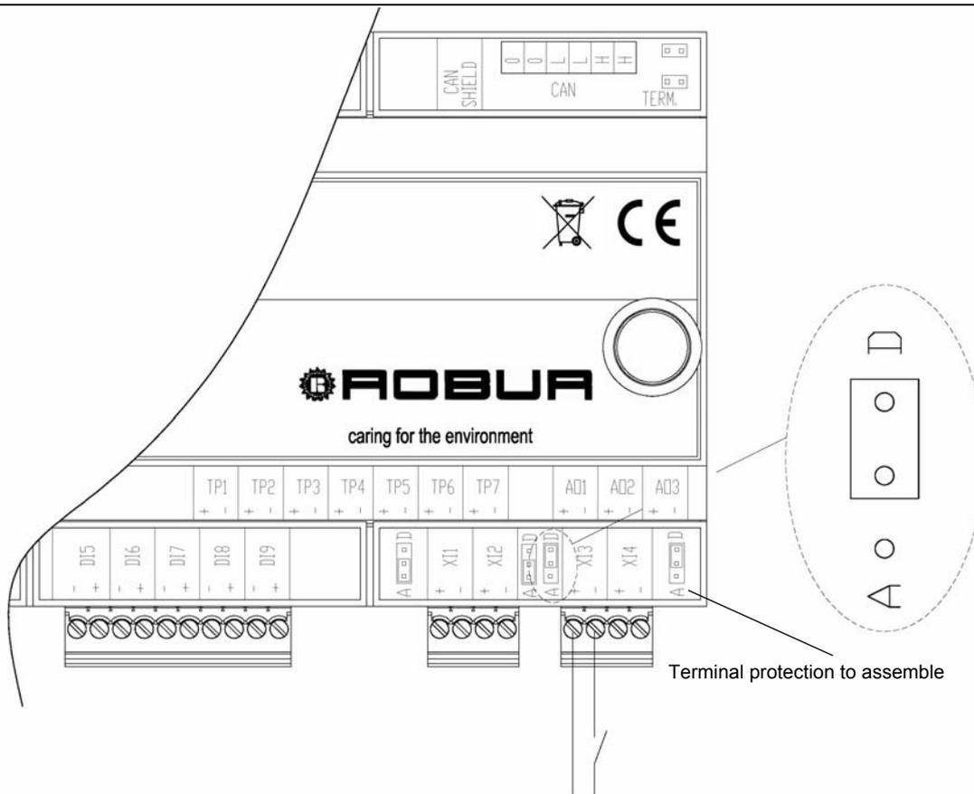
Figure 11 RB200: electrical connection for digital input
