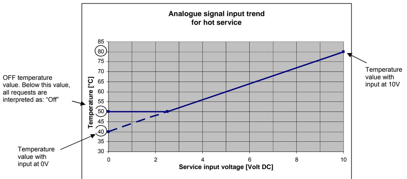
**Figure 3** Voltage signal input trend for hot analogue service (heating, DHW0 and DHW1)
