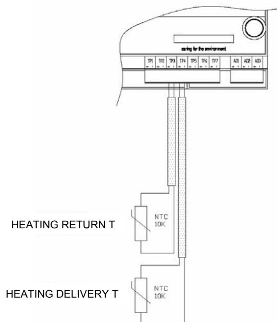
**Figure 17** RB200: Example of connection for heating manifold return/delivery sensor pair
