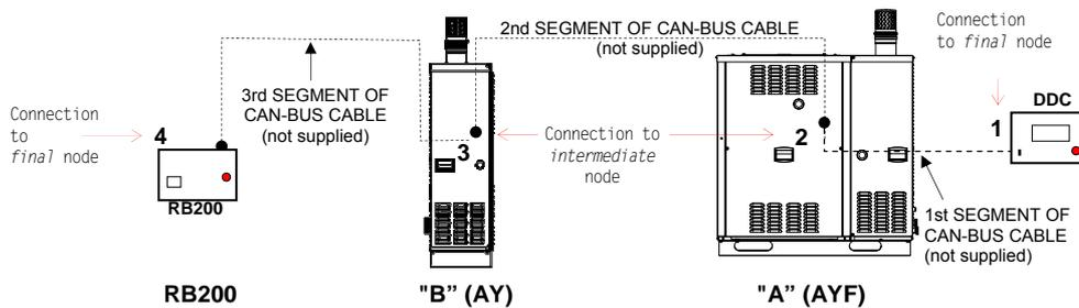
**Figure 18** Examples of CAN BUS network with 4 nodes = 2 Robur units + 1 RB200 + 1 DDC
