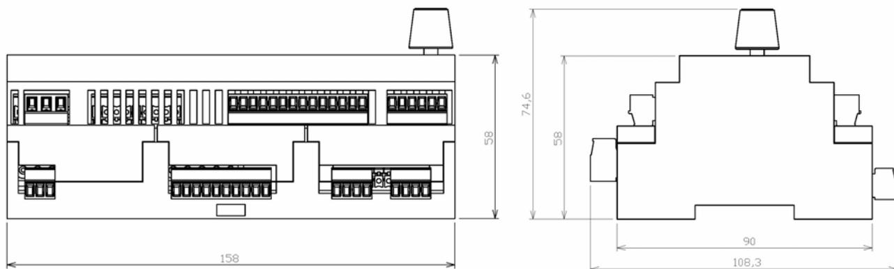
**Figure 6** Dimensions of the Robur Box series: front and side view
