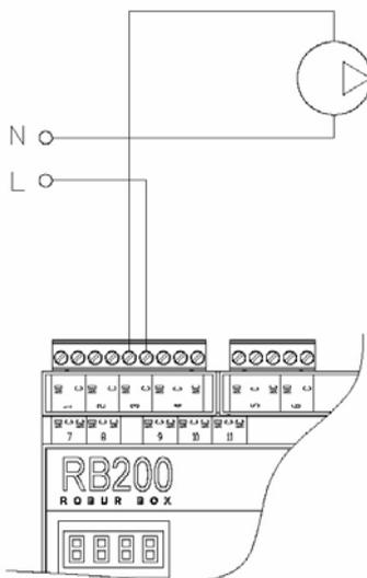
**Figure 16** RB200: Example of electric connection for circulator 3 service
