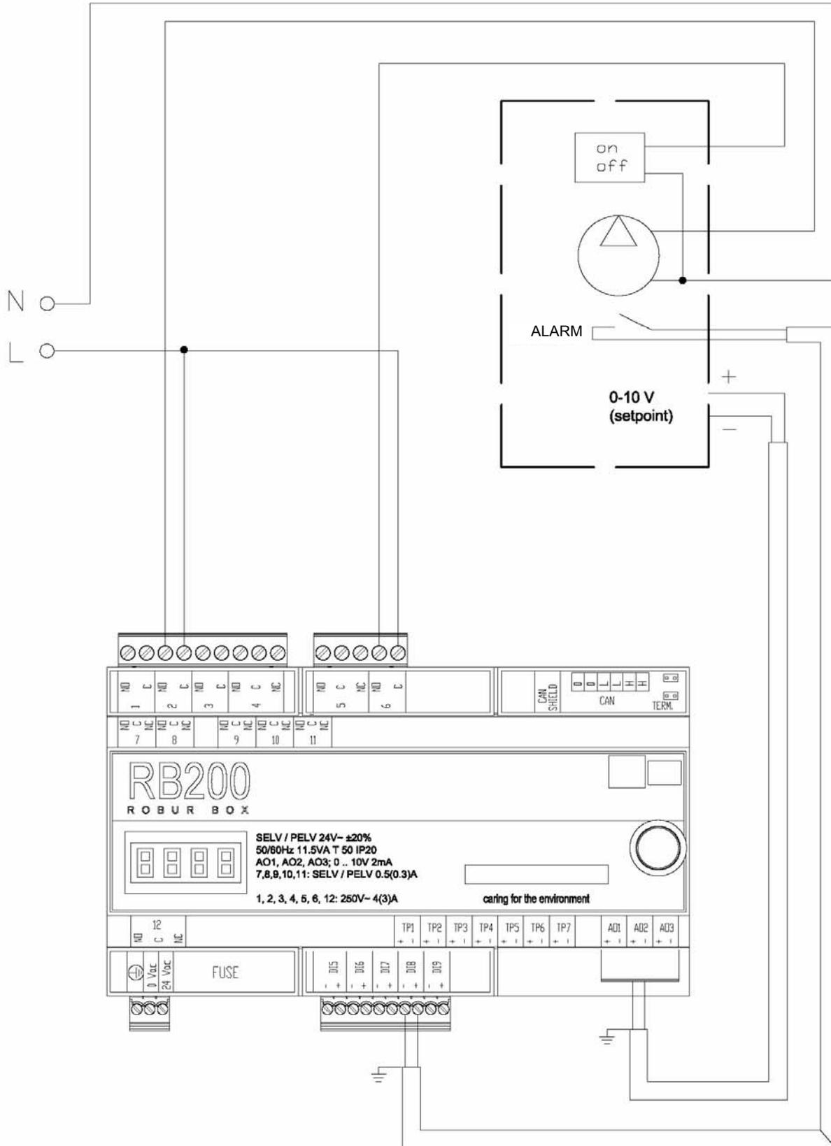
**Figure 15** RB200: Example of electric connection for generator 2 service
