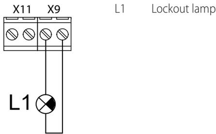
When the led comes on, in the manner described in Table 4.1 p. 26, it indicates the presence of a fault.
