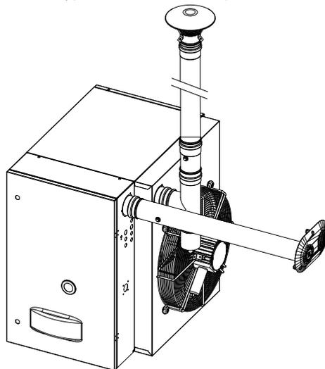
**Table 3.10** C53 type maximum allowed length with separate ducts
