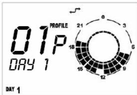
5. On the top right of the display, the word PROFILE and the number of the selected profile will appear flashing (Figure 6.5 p. 31).
