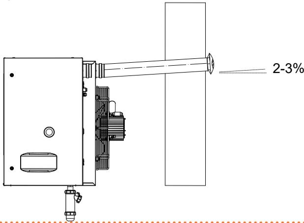
For proper installation of the wall external terminals for the flue gas exhaust and combustion air intake, follow the details given in Figure 3.8 p. 22.
