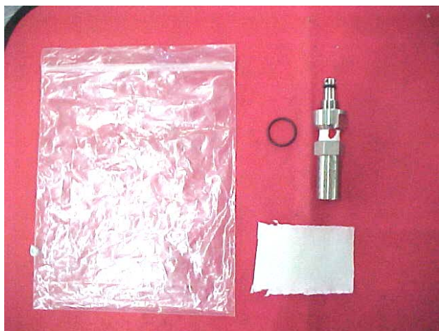
Figure 9.4 Safety valve kit - Components required for service
