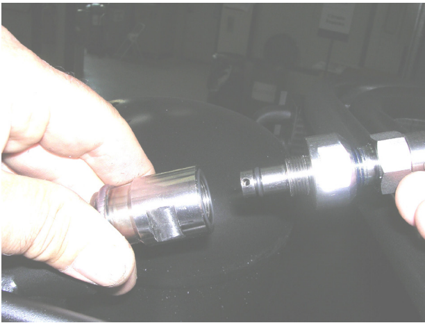
Figure 9.5 Removal of safety valve mobile part - Removal of safety valve
