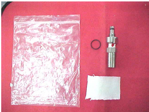
Figure 9.2 Safety valve kit - Components required for service
