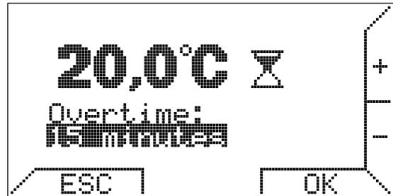
Once the duration of the overtime function has elapsed, the chronothermostat switches to the automatic operation mode. The overtime operation mode is useful when you want to interrupt the automatic operation mode by forcing a specific temperature for a specific period of time.
