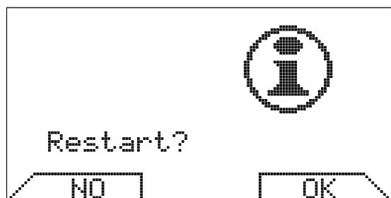
Activating the reconnection is equivalent to physically disconnecting the communications connector from the chronothermostat and then reinserting it.
