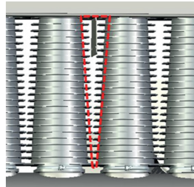
Figure 2.5 Air passage between 2 Robur exchangers
