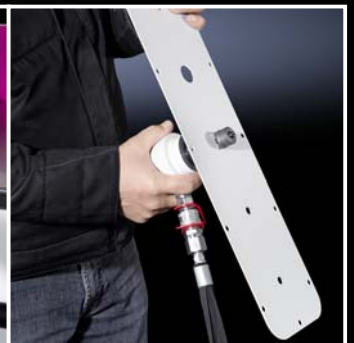
Making cut-outs in steel and stainless steel (accessories, hydraulic hose and cylinder, see page 39)
