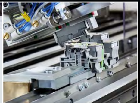
Automatic terminal block assembly
