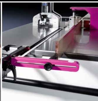
Punching busbars, pull-out measurement system
